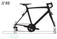
Adjust position of rear hub according to your wheel base. Place rear drop-outs on rear hub with correct rear axle adpater. Tighten your rear axle.
