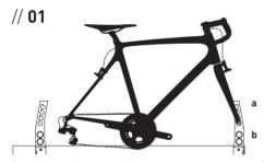
Place fork on front hub with correct front axle adapters. Tighten your front axle.
