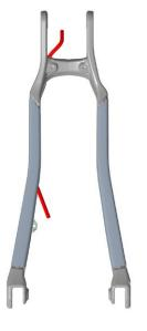
**4.** Guide the brake hose into the housing port above the bottom bracket. Make sure you insert the derailleur housing into the port labeled "Brake". Any brake port will do. a. Pic required of the port with the hose inserted into the standard port
