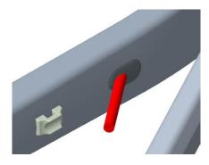
3. Push the hose forward and simultaneously twist the hose until it comes out at the forward end of the chain stay
