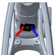
**5.** Push the cable from the rear until it appears at the head tube port. Fish it out with a pick or a bent spoke.
