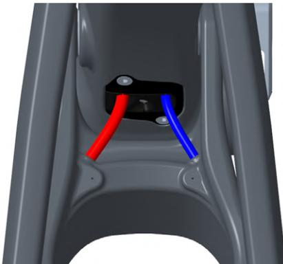
4. Push the brake hose from the rear until it comes out at the head tube port.
