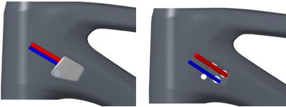
2. Push the hose forward and simultaneously twist the hose in a circular motion until it comes out at the forward end of the chain stay.
