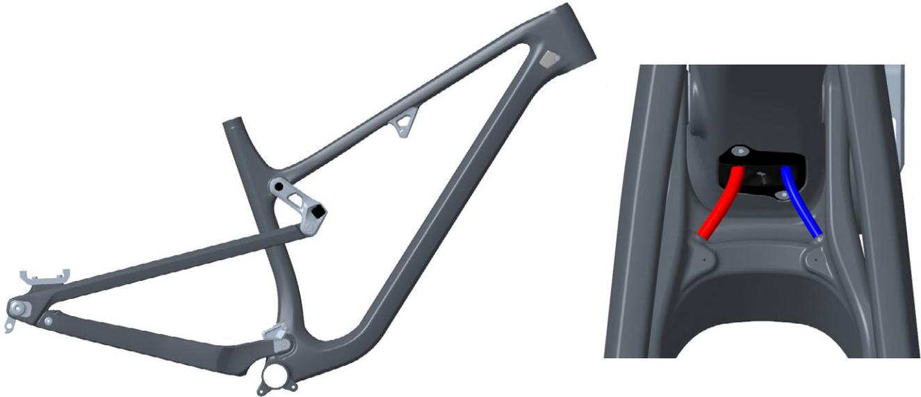
The tube-in-tube channels in the chainstay can be a tight fit, especially with the curves they have to navigate to get around the chainstay bridge. Spray soapy water or isopropyl alcohol into the opening as a lubricant to help with fitting the housing from one end to the other. Do not use grease or oil; this will leave a mess and attract dirt.
