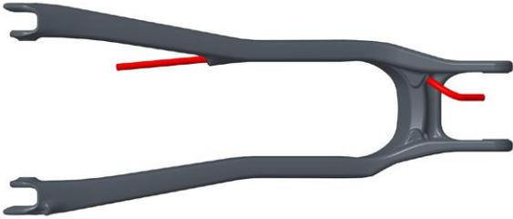
3. Guide the brake hose into the housing port above the bottom bracket. Make sure you insert the derailleurs housing into the port labeled "Brake." The standard port is the outside one, the moto / reverse port is the middle one.
