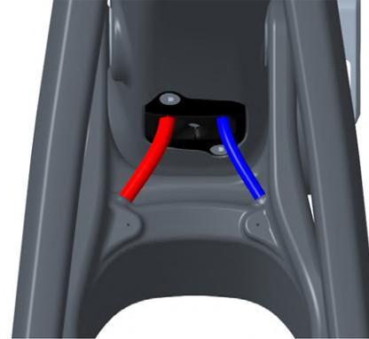
5. Push the cable from the rear until it comes out at the head tube port.
