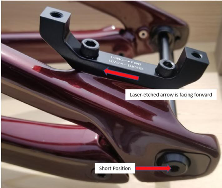
Long ----> FWD means the arrow should be pointing forward when the axle is in the long position.
