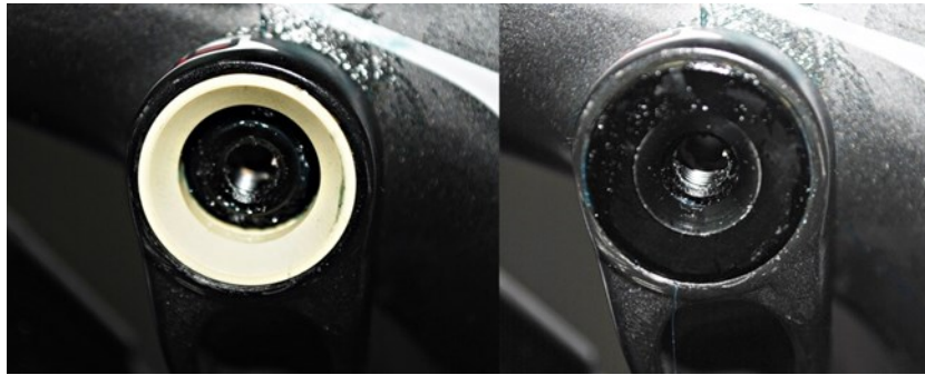
Fig. 2.8.3 Greased bushing with counter-sunk ABC washer installed
