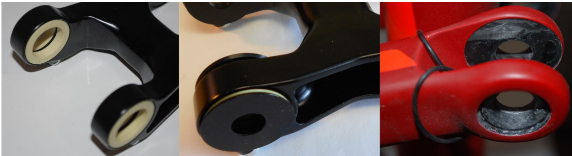
Fig. 2.11.2 Bushings pressed into the link, then greased. Washer and O-rings positioned
