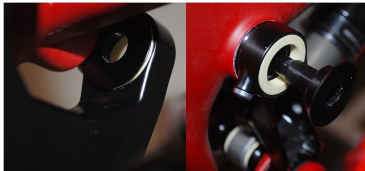
Fig. 2.12.1 Insert top tube pivot bolt from the drive side
