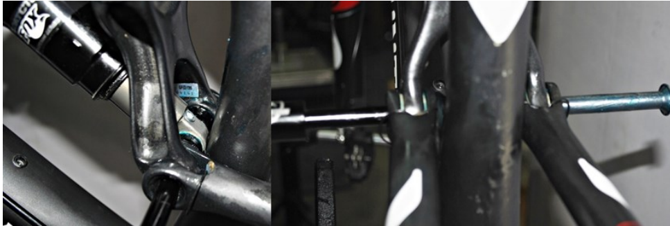
Fig. 2.7.5 Using the 9.7mm drift tool to align the seat stays with the link and shock
