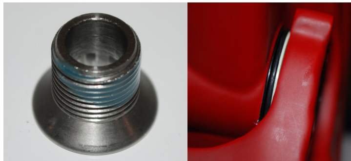
Fig. 2.10.5 Apply Loctite to the screw and torque it to 11.3 - 12.4 N-m and position O-rings
