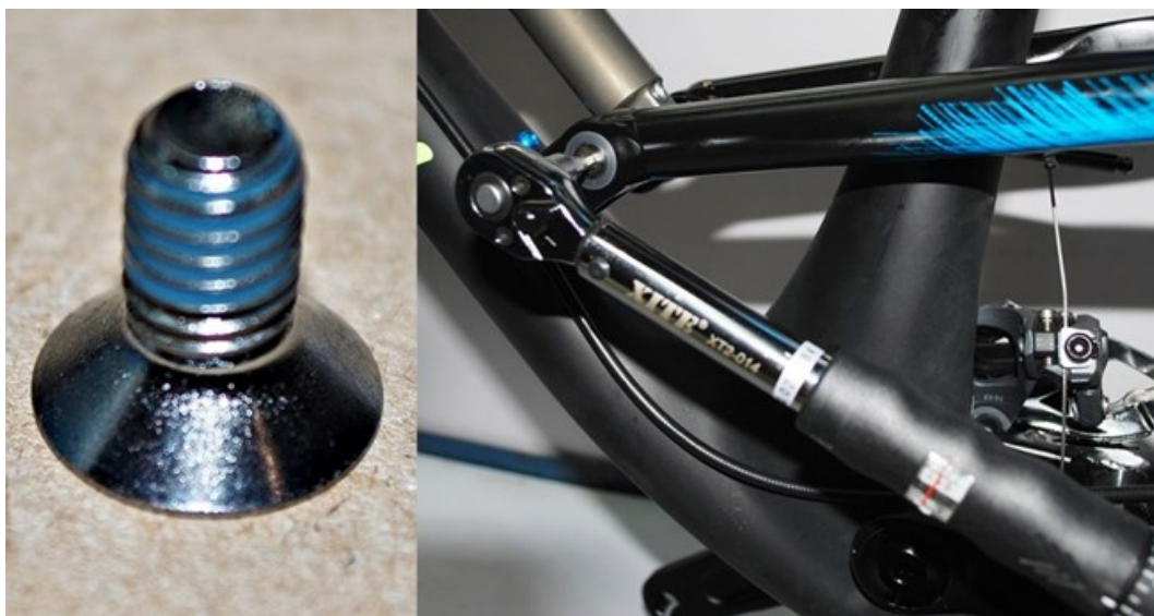
Fig. 2.3.4 Screw with Loctite and torqued to 6.7–9.0 N-m
