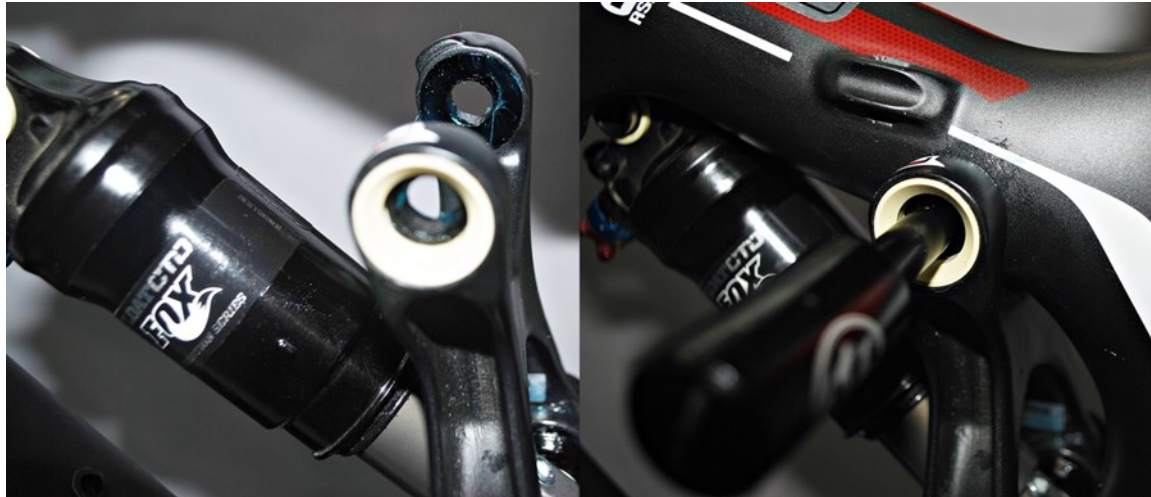
Fig. 2.8.1 Align the link with greased inboard washers using the 9.7mm drift tool
