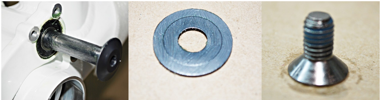
Fig. 2.2.4 Main pivot hardware
