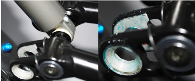
Fig. 2.4.2 O-rings positioned and greased seat stays
