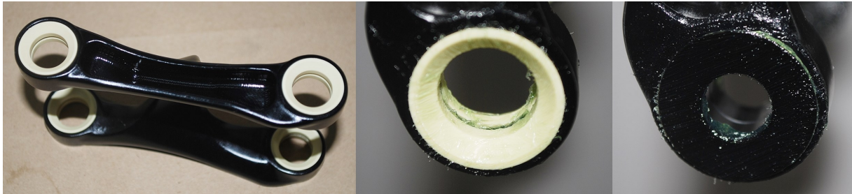
Fig. 2.4.1 Bushings presses into the link then greased and greased washer
