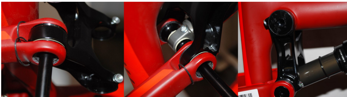
Fig. 2.11.3 Insert the pivot bolt from the drive side into the seat stay and shock
