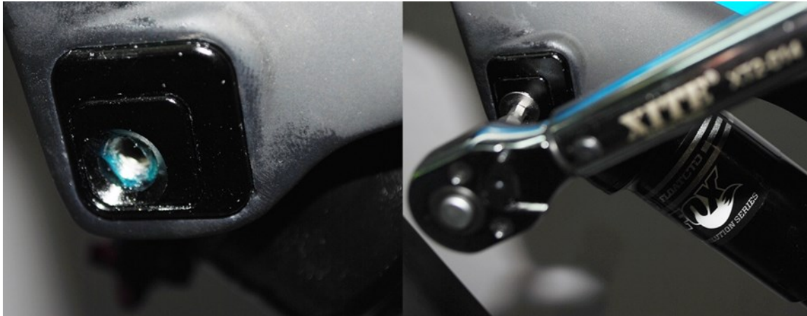
Fig 2.6.4 Grease the Ride-9 bolt threads, do not apply Loctite
