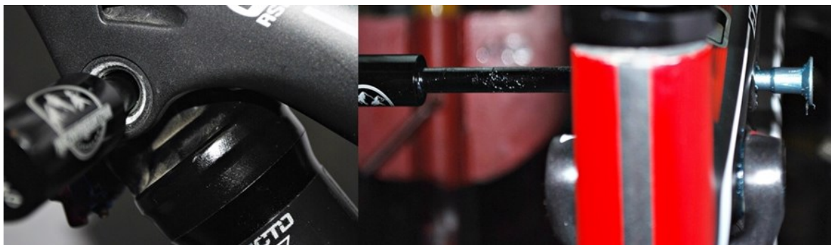
Fig. 2.9.2 Greased shock bolt inserted from the drive side
