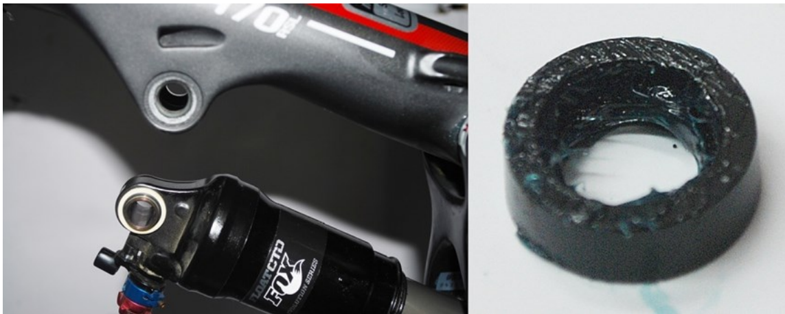
Fig. 2.9.1 Grease the forward shock spacers
