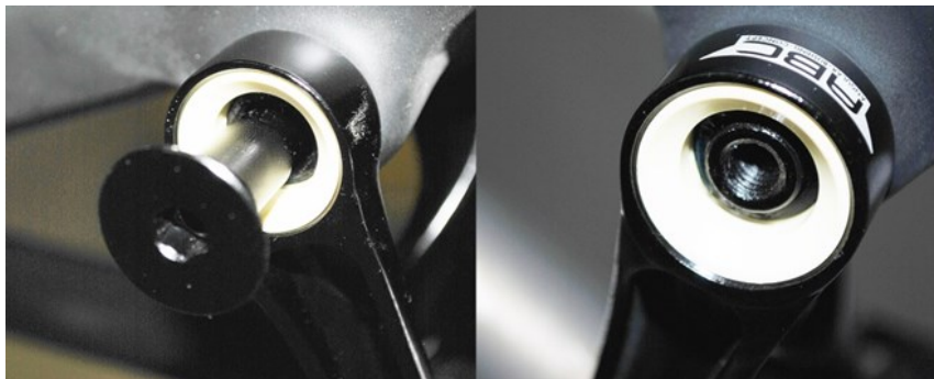
Fig. 2.5.2 Inserting the pivot bolt into the link and pivot
