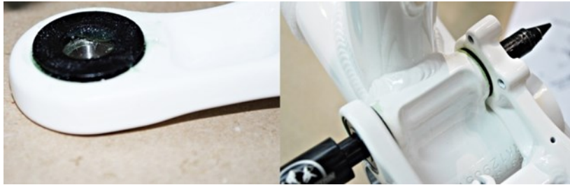
Fig. 2.2.3 Angular washer and 11.7mm drift tool
