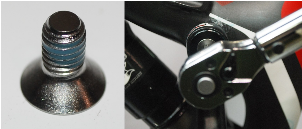
Fig. 2.8.4 Apply Loctite to the screw and torque it to 6.7-9.0 N-m
