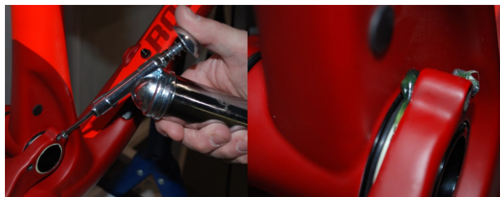
Fig. 2.10.6 Inject grease into the grease ports
