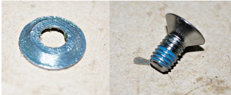
Fig. 2.1.5 Greased conical washer and LocTite coated screw
