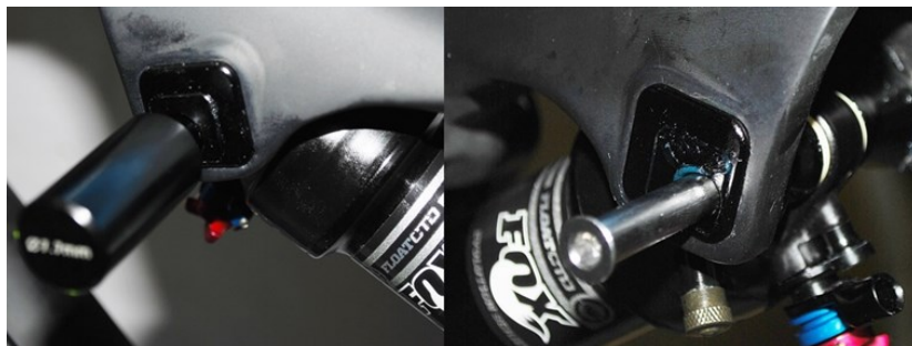
Fig 2.6.3 Using the 7.7mm drift tool to align the shock bolt
