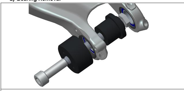
1) Using 6904 Bearing Tool Press, or a Blind Puller, remove Enduro MR17827 LLB Bearings (1807065).
