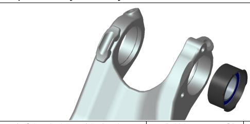
1) Orient the lobes of the Bearing Seat Sleeves as shown, so that the sleeve does not interfere with the E-Type mounting bosses.
