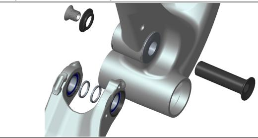
1) Grease Bearing Spacers (1807017) and the outside of the Thunderbolt Bearing Main Pivot Bolt (1807019).
