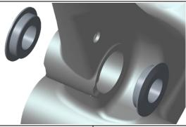
1) Using a small mallet, press in MP Adapters (1807018) into front triangle main pivot bore.
